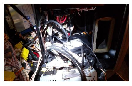
2. **1997-2006 Vision/CHXXX Models:** Mount the Base Unit behind the center of the dash. Remove the dash panels and be sure to secure the Base Unit in 2 places with zip ties.
