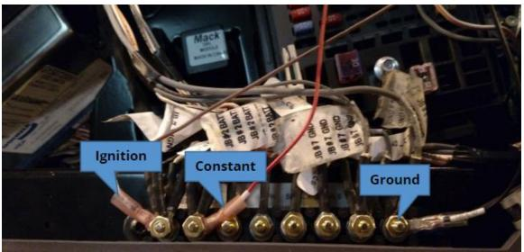
2. **1997-2006 Vision/CHXXX Models:** Power connections are all located at a power strip by the fuse panel on the right hand side of the dash.
